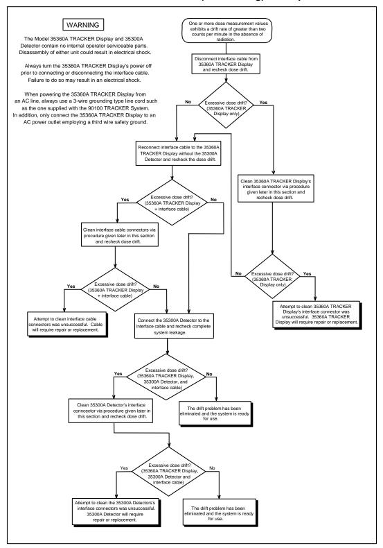
Figure 4-4. Leakage Flowchart
